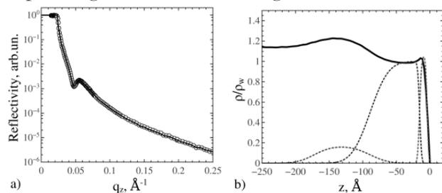
**Fig. 2.** (a) Reflectivity curve  $R(q_z)$  from the SM-30 silica sol surface. (b) Normalized profile  $\rho(z) / \rho_w$  (solid line) and model decomposition (dashed line). The data are given from [16].
