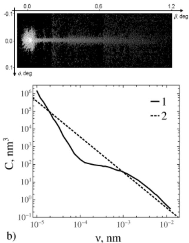
**Fig. 3.** (a) Two-dimensional distribution of diffuse scattering from the surface of TM-50 silica sol. (b) Calculated function  $C(v)$  (1) and the theoretical estimate in the frames of capillary roughness model  $C_{cap}(v)$  (2). The data are given from [17].
