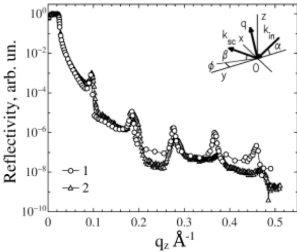
**Fig. 1.** Reflectivity curves  $R(q_z)$  measured on a DRS diffractometer (1) and an ID31 synchrotron station (2). The data are given from [21,22]. Inset: geometry of X-ray scattering from a surface.
