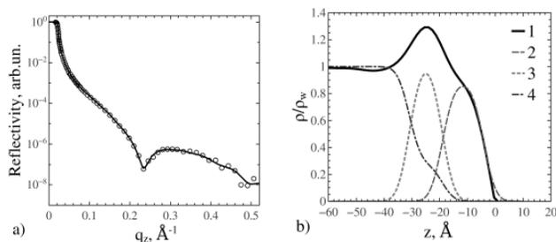
**Fig. 5.** (a) Reflectivity curve  $R(q_z)$  from the DMPS monolayer in the LC phase on the surface of the water. (b) Normalized profile  $\rho(z)/\rho_w$  (1) and decomposition of the theoretical model of MD: a layer of hydrocarbon “tails” (2), a layer of lipid polar groups (3), water (4). The data are given from [26].
