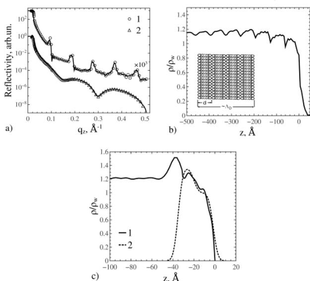
**Fig. 4.** (a) Reflectivity curves  $R(q_z)$  from DSPC film on the surface of pure SM-30 silica sol (1) and enriched in NaOH (2). (b) Normalized profile  $\rho(z) / \rho_w$  for DSPC film on the pure silica sol SM-30. Insert: lipid multilayer structure. (c) Normalized profile  $\rho(z) / \rho_w$  for DSPC film on the silica sol enriched with NaOH (1), and theoretical profile for the Langmuir monolayer of DSPC (2). The data are given from [21,22].
