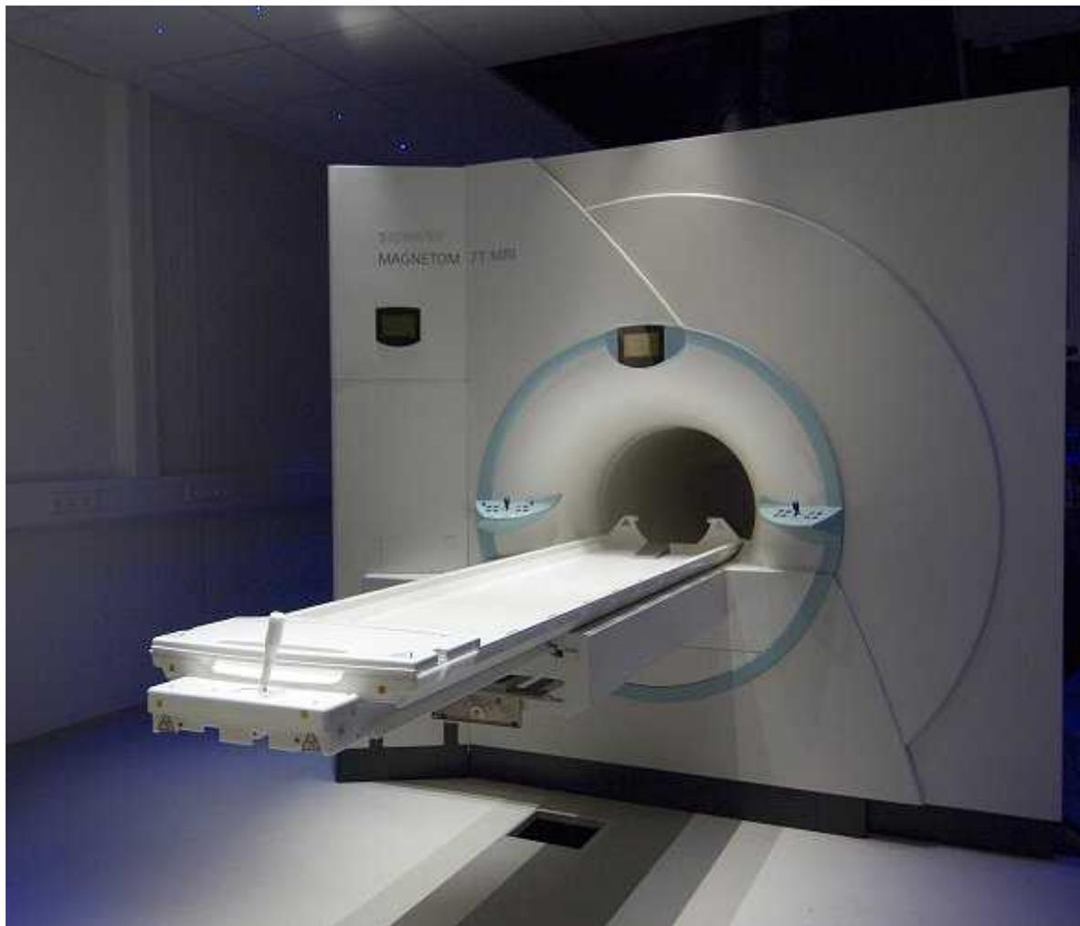
7 T MRI system with a superconducting 32-ton magnet
